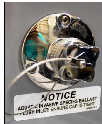
Ballast tank flush kit port, located on starboard side of the transom.
