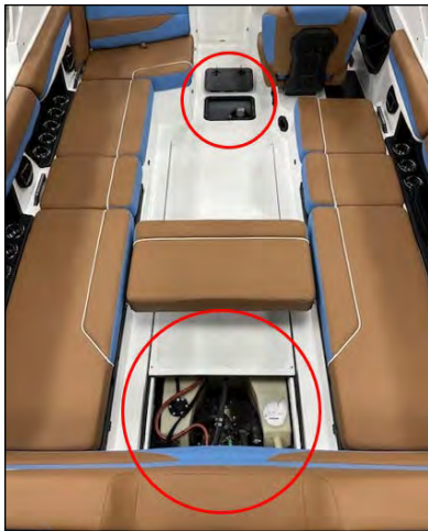
Fill pump valves and bilge T-handles are accessible through the fore and aft access panels (shown above, circled in red).
