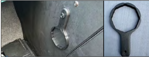
Sea Strainer Location and Removal Tool.
