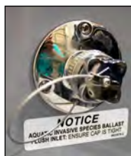
Ballast tank flush kit port, located on starboard side of the transom.
